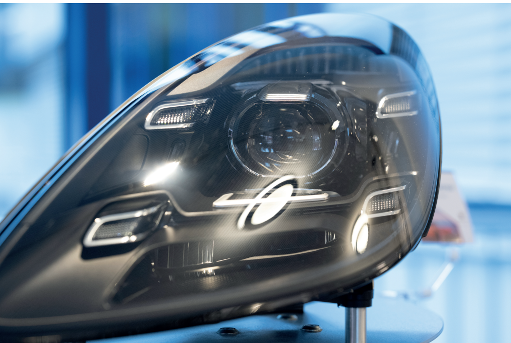
A modern headlamp consists of up to 300 individual parts that must be assembled and positioned with high precision. © Zeiss/ZKW
