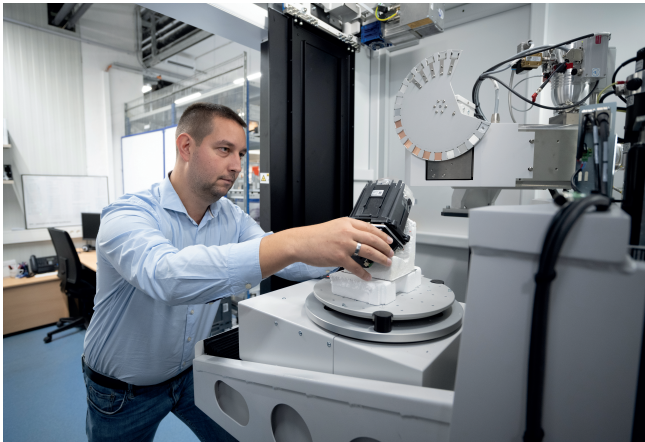
Martin Janisch clamps a lighting module into the Zeiss Metrotom 1500 in the measuring laboratory. © Zeiss/ZKW
